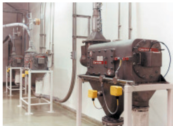
In-line sifter placed directly in lean phase pressure or suction conveyor.
