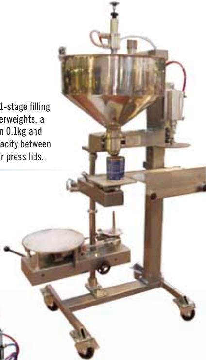
Filling machine type 2000 with closed filling head, 2-stage filling actuator for coarse and fine filling, electronic weighing system (available in both explosionproof and non explosionproof design) and pump for the product infeed. In standard design, the filling method is above level filling. Subject to the type of product, below bughole or submerged filling methods are also available.
