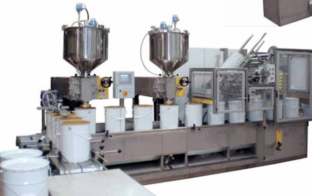
Fully automatic volumetric filling machine type V230i-Twin with two 20l dosing units suitable to fill metal and plastic pails with volumes between 0.5l and 20l in one shot. The two dosing units can be used to separate non-compatible products or for higher speeds if e.g. 50% of the pail is filled with the first head and 50% with the second head.
