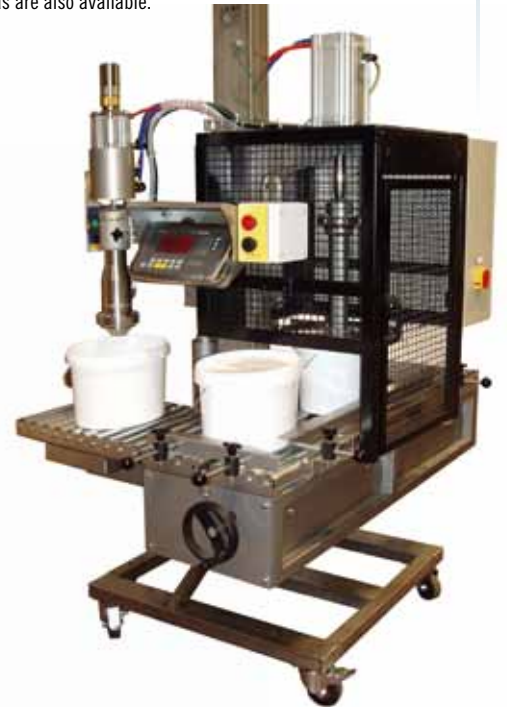
Filling machine type 232 with closed filling head, 2-stage filling actuator for coarse and fine filling, electronic weighing system (available in both explosionproof and non explosionproof design), non driven conveyor at the filling position and mini transport system to bring the filled containers automatically to the lid closer station. The lid closer station can handle both press lids and crimp lids. In standard design, the filling method is above level filling. Subject to the type of product, below bughole or submerged filling methods are also available.
