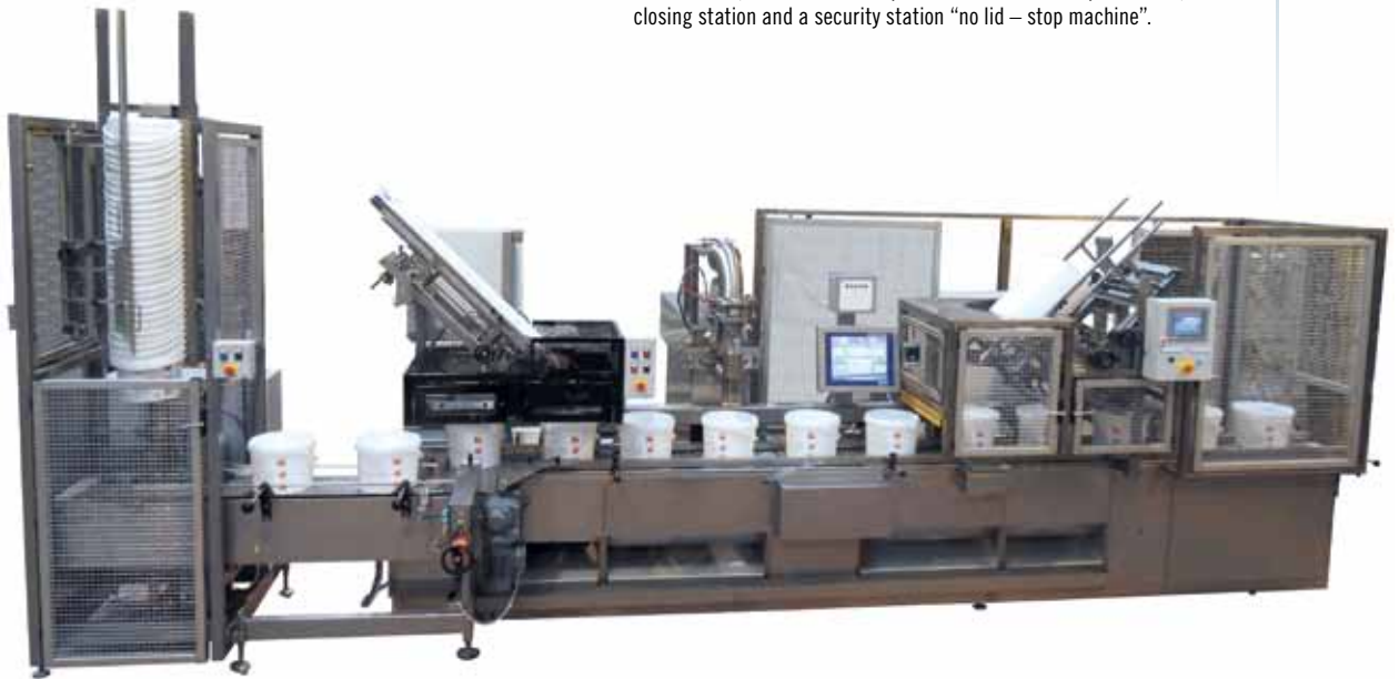
Fully automatic volumetric filling machine type V302P, shown here in a design with pail denester for plastic and metal conical pails, a special "pot denester", a volumetric filling station, immediately followed by a checkweigher which stops the machine if any under- or overfilled cans are detected, an automatic lid placer for metal and/or plastic lids, a lid closing station and a security station "no lid – stop machine".
