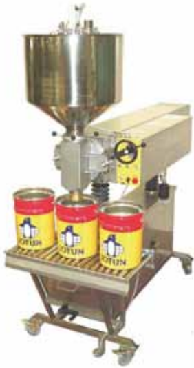
Filling machine type Vreebase DU02 with dosing mechanism suitable for fills between 0.5l and 20l in one dosing shot, adjustable in height, and presenting table designed as a 1 m long non driven conveyor mounted at a fixed height.
