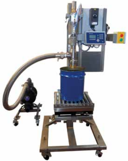
Filling machine type 2000 with closed filling head, 2-stage filling actuator for coarse and fine filling, electronic weighing system (available in both explosionproof and non explosionproof design) and pump for the product infeed. In standard design, the filling method is above level filling. Subject to the type of product, below bughole or submerged filling methods are also available.
